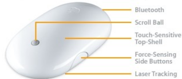
Key features of the wireless Mighty Mouse
